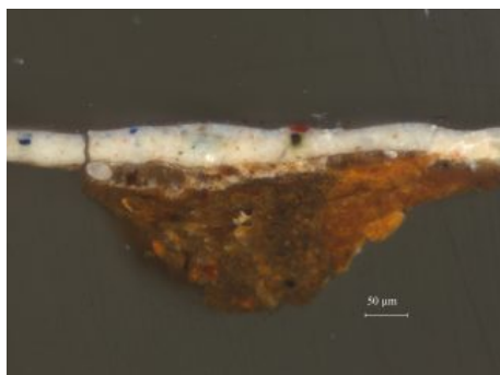
Fig. 26 Cross-section (MH1126x02) from Willem Kalf, Still Life with Fruit and Wineglasses on a Silver Plate (fig. 25), showing a lower ground layer of yellow and brown earth with fine black and a few lead white particles, and an upper ground layer of yellow earth, lead white and fine black, 200x magnification, bright field illumination
