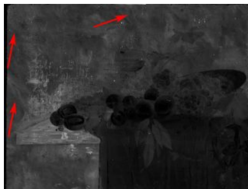
Fig. 16 MA-XRF map for iron (Fe-K) from Johannes Rosenhagen, Fruit Still Life (fig. 13), showing the application of the background in diagonal brushstrokes (indicated with red arrows)
