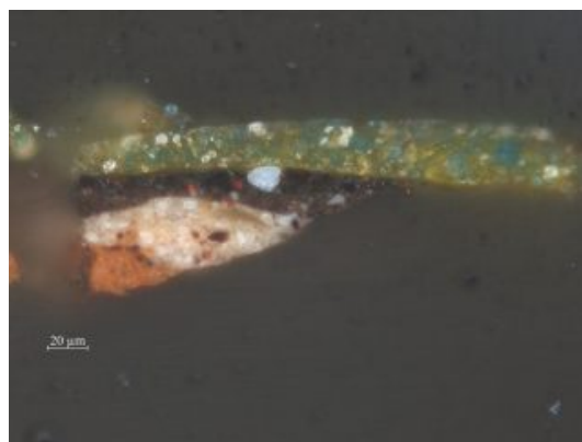
Fig. 34 Cross-section (MH1099x03) from Jan Davidsz. de Heem, Vase of Flowers (fig. 33), showing a lower ground layer of red earth and an upper ground layer of lead white and earth pigments, 400x magnification, bright field illumination
