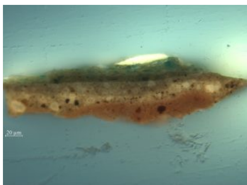
Fig. 32 Cross-section (MH0049x02) from Jan Davidsz. de Heem, Garland of Fruit and Flowers (fig. 30), showing a lower ground layer of red earth and an upper ground layer of lead white and earth pigments, 400x magnification, UV fluorescence
